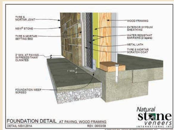
Foundation Detail at Paving, Wood Framing
